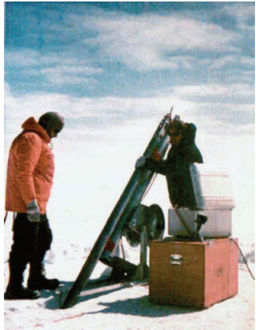
Fig. 9.2 Sigfus Johnsen and Steffen Hansen tilting the shallow drill into vertical position.
