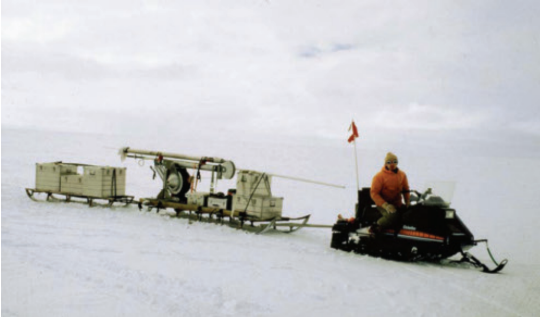
Fig. 9.3 Steffen Hansen on a snow mobile pulling two Nansen sledges with the entire drill equipment including fuel, generator packing materials, radio emitter and other emergency accessories.
