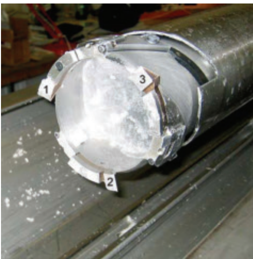
Fig. 14.5. Only in early July, the drill came up with a well sized ice core in the core barrel. The cutter knives, are numbered 1, 2 and 3. Photo: Lars Berg Larsen.
