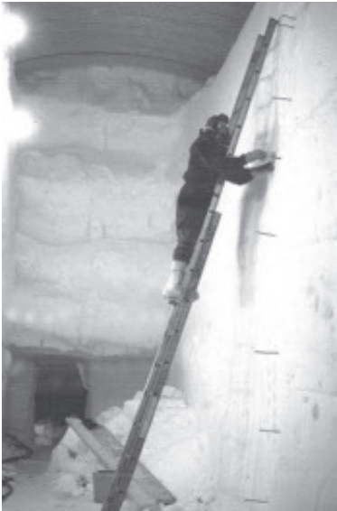
Fig. 5.5 WD cutting samples from a 5 m high snow wall. The sticks mark summer layers estimated from melt layers. This profile reached back to 1953.
