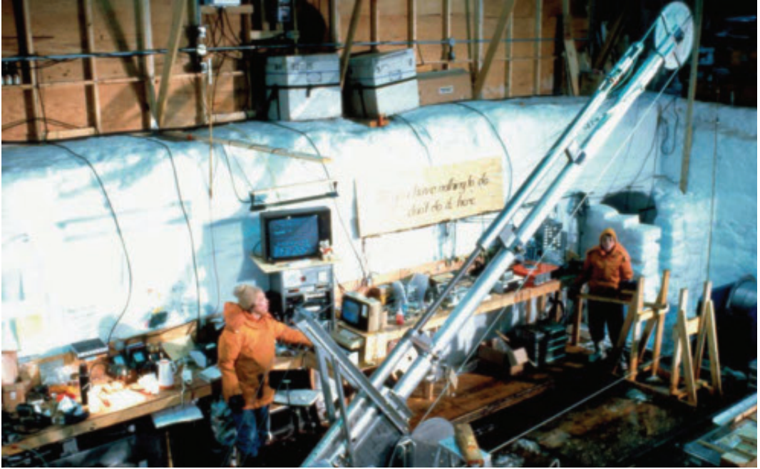
Fig. 10.2 The drill ball. ISTUK is being tilted by a hydraulic pump system.
