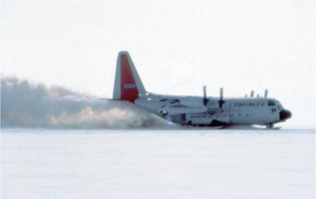
Fig. 12.1 After unloading 10 tons of goods, a chartered US Air Force Hercules takes off using jatoes.
