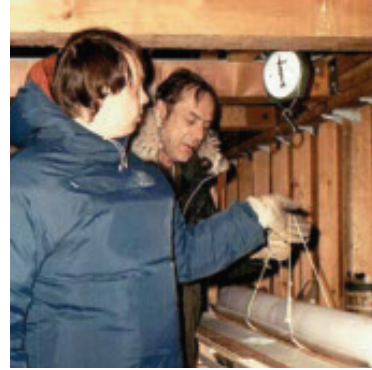
Fig. 7.4 Sifus Johnsen and Chester Langway measuring the density of an ice core increment. The density increases downward from 350 \text{ kg/m}^3 at surface to 920 \text{ kg/m}^3 at a depth of c. 100 m, where the snow has been compressed into solid ice.
