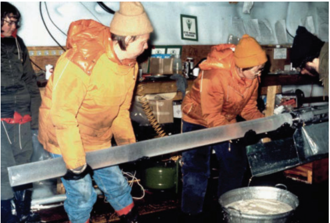
Fig. 10.3 An ice core from great depth is released from the core barrel. Note that it is transparent. The air bubbles are dissolved in the crystal lattice at great pressures. When the ice relaxes at normal pressure they re-appear, but now around micro-particles that occur most frequently in summer layers. Thereby these layers become visible and may be used for dating by counting summer layers downward.
